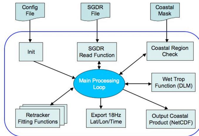
**Figure 1: Process and data flow in the COASTALT Baseline processor**
